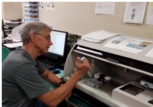
Research Scientist at the DEP's Bureau of Freshwater and Biological Monitoring performs toxin analysis using a Cyanotoxin Automated Assay System. Source: DEP.
